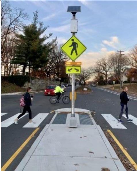
A *pedestrian refuge island* is a refuge area that is intended to help protect pedestrians crossing a road, providing a place to wait as vehicular traffic passes. This pedestrian refuge island in Arlington features *Rectangular Rapid Flashing Beacons (RRFBs)*, which further alert motorists that a pedestrian is crossing the street. When a pedestrian approaches the crosswalk, they press a button that activates a set of flashing lights, improving their visibility as they cross the street.
